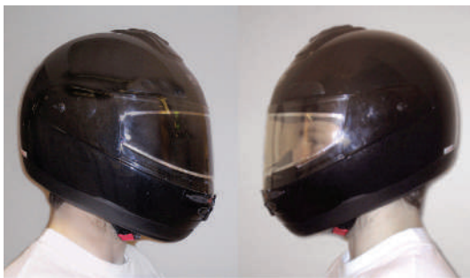
Figure 2 Motorcycle helmet with visor based on electrochromic foil, in dark and transparent state.
