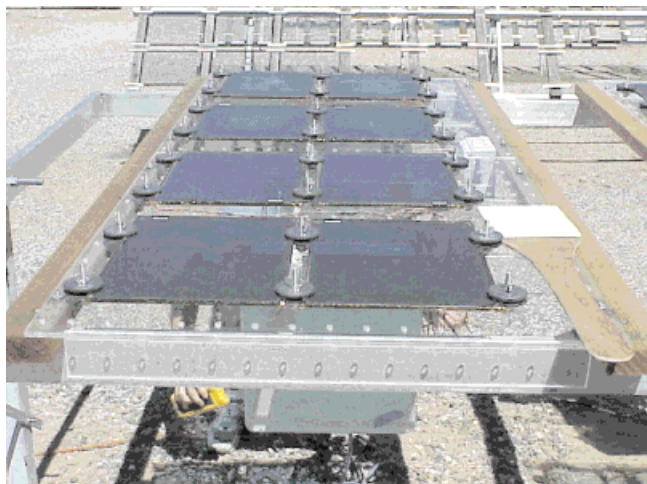
Fig. 2. Gentex windows being tested in Florida. A man is visible beneath the nearest.
