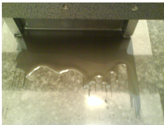
Figure 4.3: The slurry was contracting on the plastic film during tape casting with the doctor blade.[Picture: Morten Onsrud]
