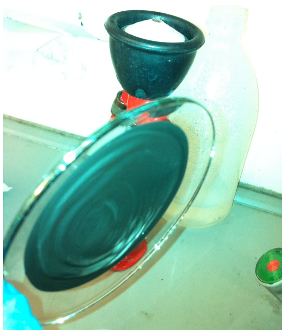
Figure 5.1: The watch glass with the slurry after about 27 hours of air exposure. [Photo: Marius Uv Nagell]
