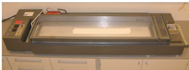
Figure 3.2: This is the tape caster with a doctor blade used in the project. [58]
